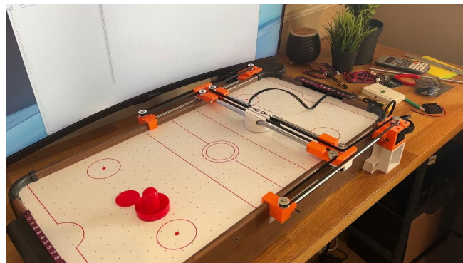
Air hockey bot with CoreXY gantry (credit: zershot)
