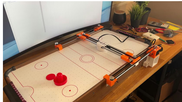
Air hockey bot with CoreXY gantry (credit: zeroshot)
